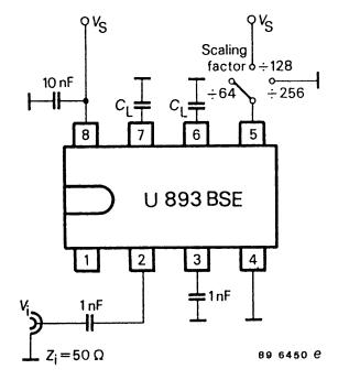
C<sub>L</sub>=Total capacitive output load including test fixture and test epuipment capacitance
